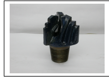
Step Type Bit with 2-3/8" API-Reg Threads
